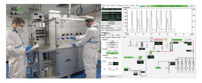
On the left, completed installation of CordenPharma's SFC 1500 (PIC Solution) technology for lipids purification at CordenPharma Chenôve. On the right, a screenshot of successful first injections towards highly pure lipid GMP manufacturing using the new SFC technology and process.
