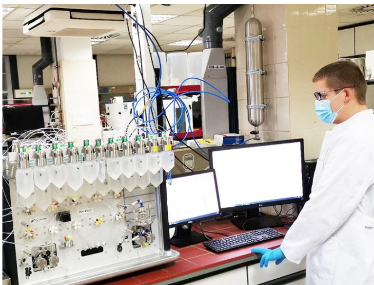
Elongation monitoring using PeptiSystems' PeptiPilot during the synthesis of GLP-analogue at CordenPharma's Peptide Centre of Excellence (Frankfurt, DE).
