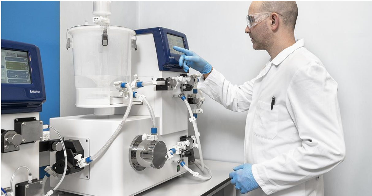
[Photo by CordenPharma] Lipid NanoParticle (LNP) Purification Process Development and Scale-up via Tangential Flow Filtration (TFF)
