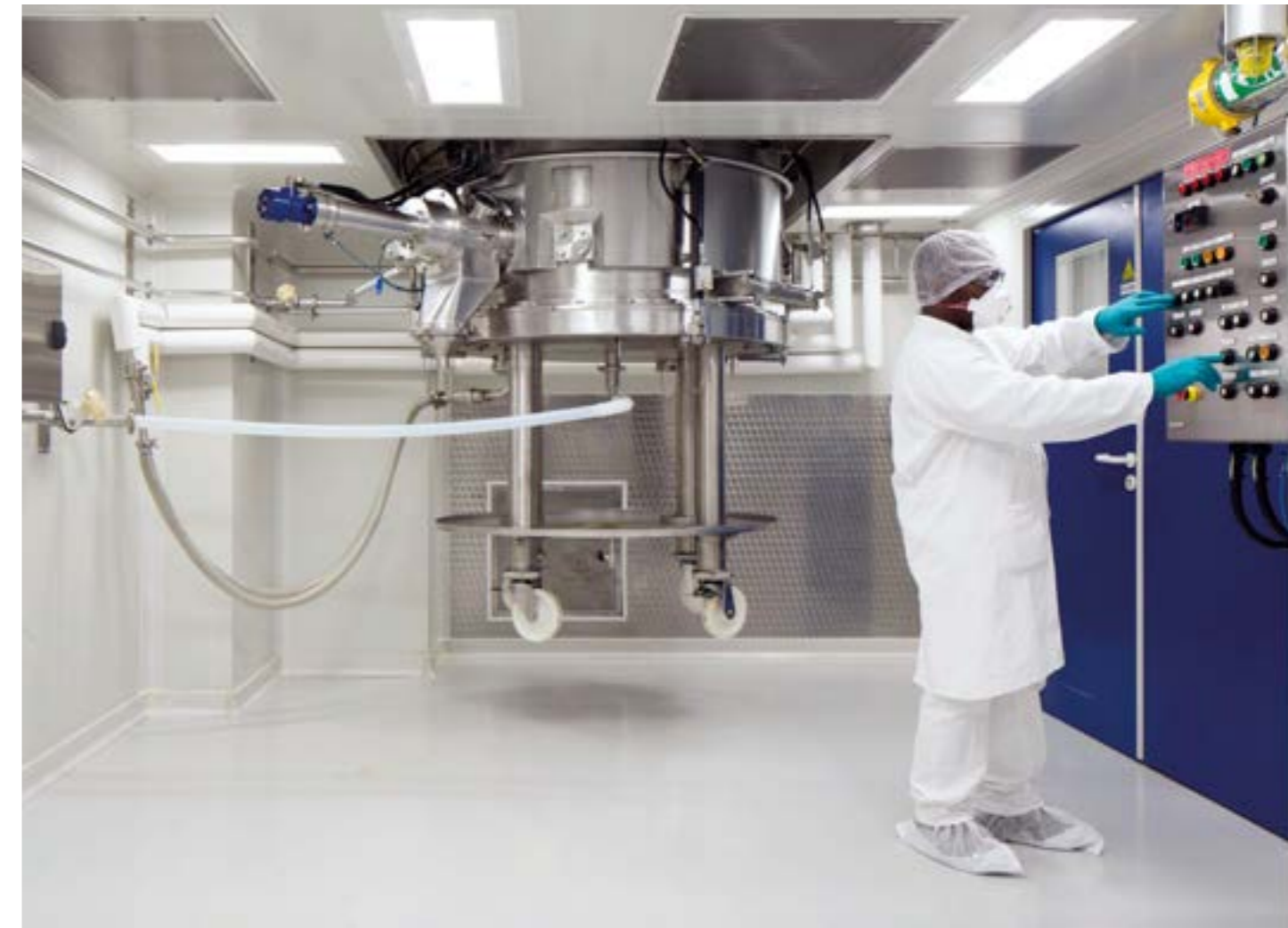
Drying of the final crude API in a filter dryer at CordenPharma Brussels (BE).
