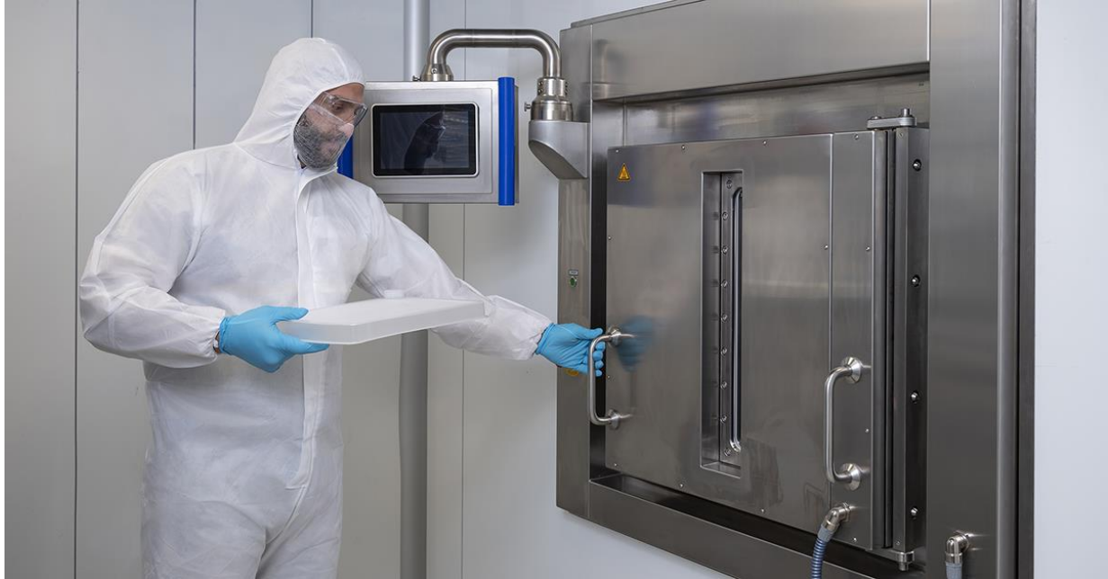
[Photo by CordenPharma] Freeze drying isolation of APIs in the containment area of CordenPharma Frankfurt (DE).
