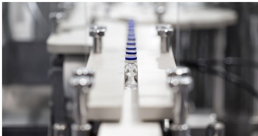
[Photo by CordenPharma] – Aseptic vial filling line in CordenPharma Caponago, Italy.
