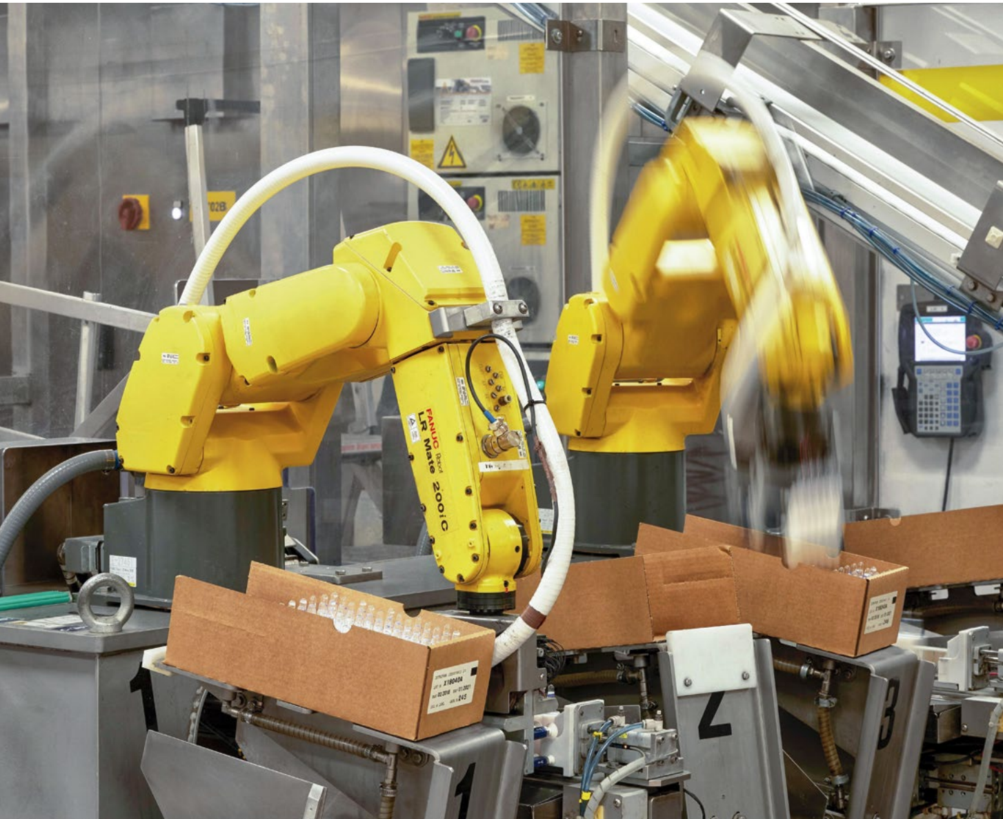
Fully-automated packaging line at CordenPharma Caponago (IT).
